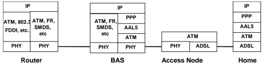
Figure 7. Protocol Stack for PPP Terminated Aggregation
