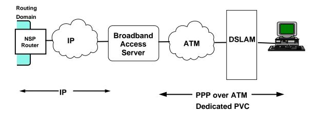
Figure 6 - Network Topology for PPP Terminated
