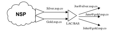
Figure 10. Logical Downstream Partitioned by the NSP
