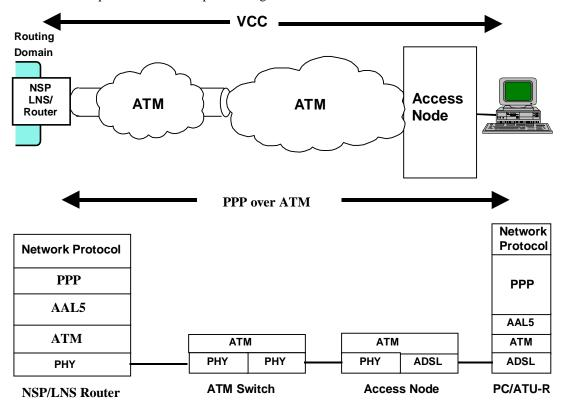
Figure 4 - Transparent ATM Core Network
