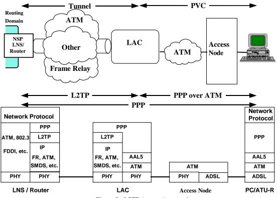
Figure 5 - L2TP Access Aggregation
