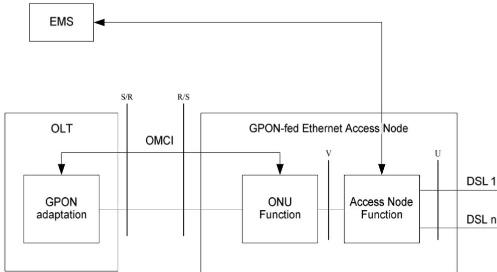
Figure 8 – Configuration Management for GPON-fed Ethernet Access Node
