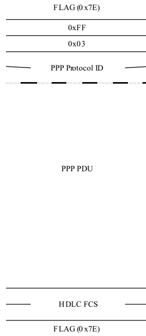
Figure 5-1: HDLC-like-framed PPP PDU
